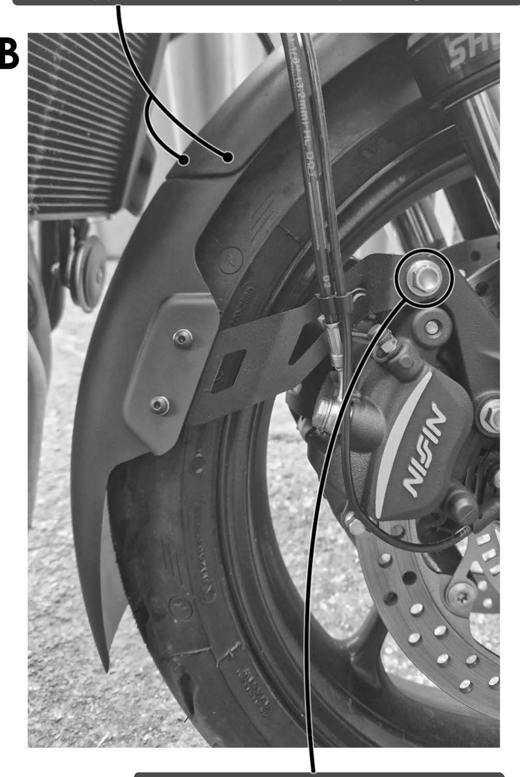
Remove this brake caliper bolt on each side of the bike. Refit the bolt with the mudguard brackets in place as shown here.
