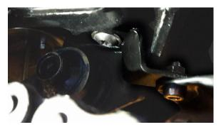
A *%*" drive ratchet with short extension bar and 10mm socket along with a stubby pozi-drive screwdriver will be helpful in removing and re-installing the two forward mounted chain guard fixing bolts.
