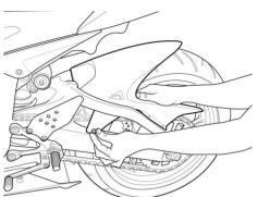
**4** Secure the hugger in place using the Three original fixing points and bolts removed in step **1**.
