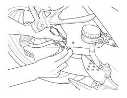
**6.** Fix the lower protection arm away from the tyre using the zip tie provided.
