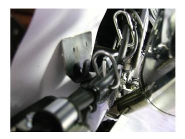
using the M6 x 20mm bolt supplied, refit the brake hose guide to the tab, fully tightening the bolt, which should pass through the single hole in the bracket. Secure the bracket to the tab with the Nyloc nut and steel washer supplied to the rear of the bracket. Fully tighten.
