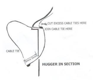
Position the hugger, carefully pass the cable ties through the swing arm unit hole. Fasten the cable ties without fully tightening at this stage.
