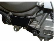
Remove both 10mm bolts securing top of oil radiator to fixing bracket on bike (one each side top of exhaust) and insert supplied big bracket marked "A" facing forward from behind oil rad to line up all holes, trapping new bracket between original bracket behind, and existing rubber washers in front. When all is lined up and new bracket is seated upright behind oil rad replace both 10mm bolts and tighten.
