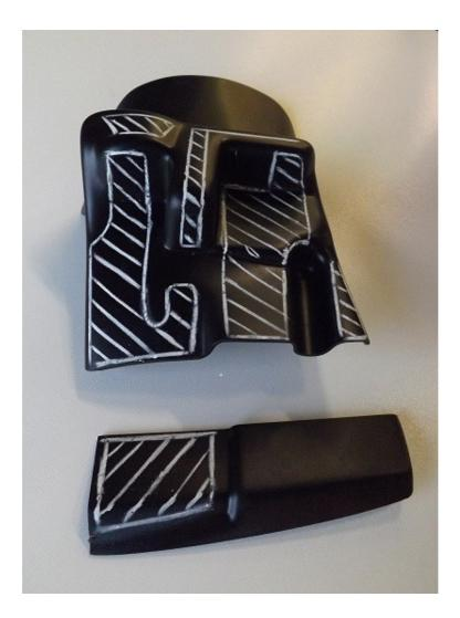
You may wish to mask the areas immediately adjacent to the parts being fitted in order to reduce the risk of contamination from excess adhesive. Any excess adhesive should be left in place until it is fully cured and then it can be removed cleanly. First use a knife to cut through the glue at the point where it protrudes from the back of the part. Then simply peel away the rest of the excess adhesive.
