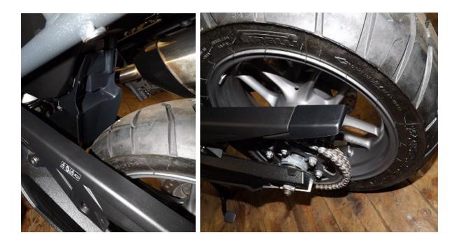
Both items are attached using the 'No Screws' adhesive supplied. No additional mechanical fixings are required. It is recommended that all work be carried out at or above 12 degrees Centigrade.
